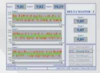
The DELTA MASTER 3 graphic visualisation and operation interface allows production motoring tailored to the setpoints and tolerances of the individual products. The Product Management option offers simple management of the individual products with regard to nominal thickness, tolerances and other settings for every measuring point. The programmable storage of measuring results allows
