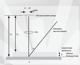
contact up to 50 times per second at any sheet speed even on difficult surfaces on which conventional spot laser triangulation sensors fail due to the surface structure. The DELTA MASTER sensor determines the material thickness from the distance between the sensor and the material surface. Various calibration, difference and compensation methods guarantee accurate and stable measurements even under harsh industrial conditions.
