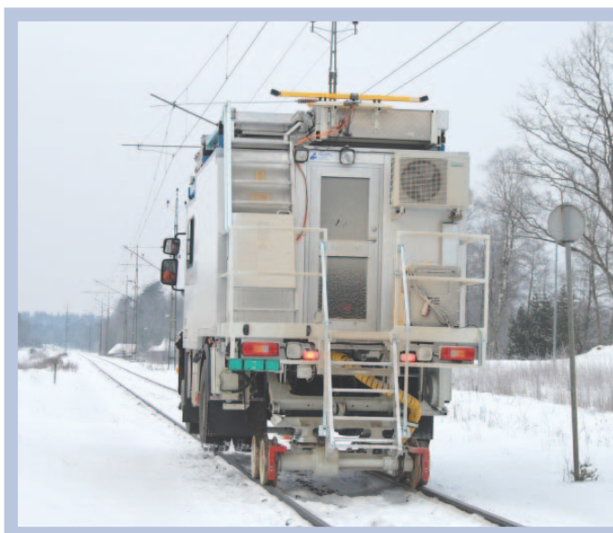
Fig. 1: The OVHWizard measuring system on a road-rail vehicle
