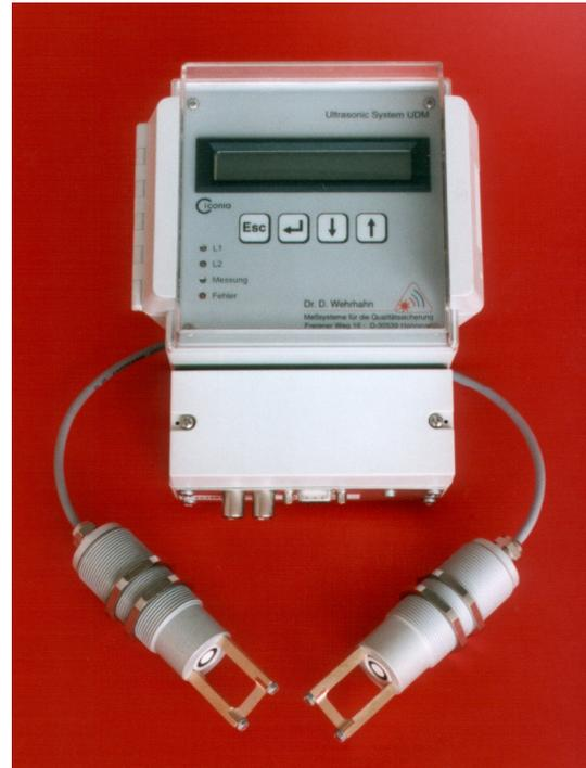
The ultrasonic distance measuring systems **UDM 1000** and **UDM 2000** facilitate highly accurate distance and thickness measurements in gaseous mediums on resonating surfaces, such as metals, glass, wood, liquids and many types of fabric. Whereby measuring accuracy amounts to up to  $10\mu\text{m}$ !
